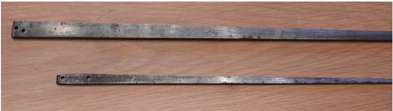
Figure 3: Close-up of NPU reamers showing characteristic prick punch marks and rivet holes
