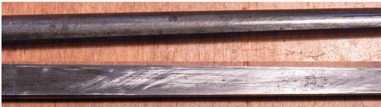
Figure 6: Composite photo – two views of O'Mealy Reamer #2 (D section) showing prick punch marks and edge relief
